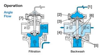
A Hydraulic Command [1], which pressurizes the Upper Control Chamber [2], forces the Diaphragm [3] actuated Plug Assembly [4] to move towards the Supply Port Seat [5], eventually sealing it drip tight. This allows flow from the filter through the Drain Port Seat [6]. Venting the upper control chamber causes the line pressure, together with the Spring [7] force, to move the Valve back to filtration mode.
