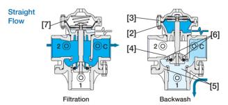
A Hydraulic Command [1], which pressurizes the Lower Control Chamber [2], forces the Diaphragm [3] actuated Plug Assembly [4] to move towards the Supply Port Seat [5], eventually sealing it drip tight. This allows flow from the filter through the Drain Port Seat [6]. Venting the upper control chamber causes the line pressure, together with the Spring [7] force, to move the Valve back to filtration mode.
